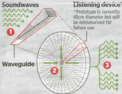
**2** The soundwaves meet in the middle, where they are combined into a single wave
